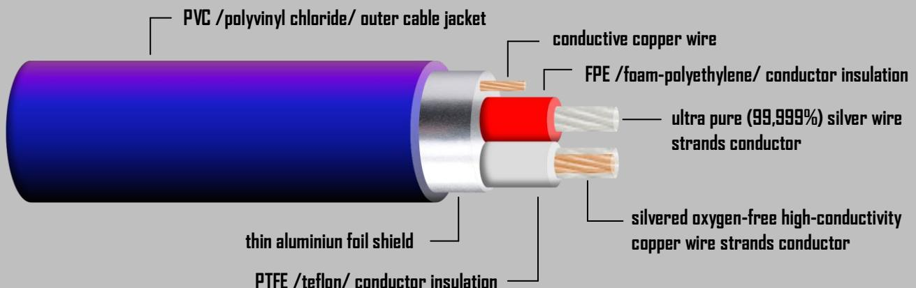
Desire HYBRID is designed to unite the best features offered by ultra pure silver and high-conductivity copper in one single cable. The result is a fast signal transfer with focus on detail, micro-dynamics, „hand in hand“ with „smoothness“ and „sovereignty“.
