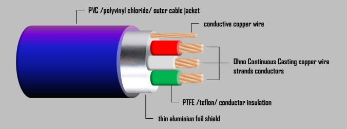
Desire CORE is an emphatic mid-level runner that is using ultra pure copper coated in "Ohno Continuous Casting" (OCC) process. OCC process creates almost perfect metal surface which can be seen in mono-crystalline materials. Use of this coating leads to rapid increase of signal transmission and lowers electrical resistance.
